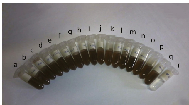
Fig. 6. Photograph of a series of eppendorf tubes with Bi NPs in water with 3.5 mM of different amino acids. From the left to the right: (a) pure colloid; (b) leucine; (c) valine; (d) tyrosine; (e) phenylalanine; (f) histidine; (g) glycine; (h) isoleucine; (i) aspartic acid; (j) methionine; (k) threonine; (l) serine; (m) glutamic acid; (n) arginine; (o) asparagine; (p) glutamine; (q) proline and (r) cysteine.
